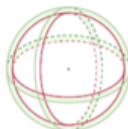
Figure 2: Each of the spheres has a volume V corresponding to respectively r = r + dr (green) and r = r (purple). The element dV is the region in space enclosed by these two spheres.
